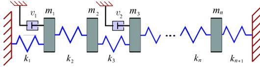
Fig. 1. An  $n$ -mass oscillator with two dampers, and different viscosities.
