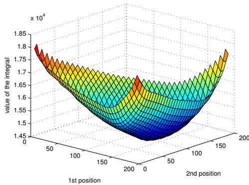
Fig. 2. x and y-axis: positions of the two dampers, z-axis: value for the minimal value of the integral (3).
