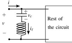
Fig. 3. LC tank formed upon shorting of the port
