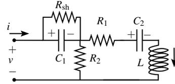
Fig. 5. A capacitor with a shunt  $R_{sh}$
