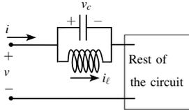
Fig. 2. LC tank in series with the port
