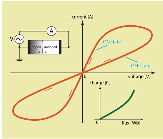
Fig. 3. Current-voltage plot demonstrating hysteretic phenomena of HP Lab's device.
