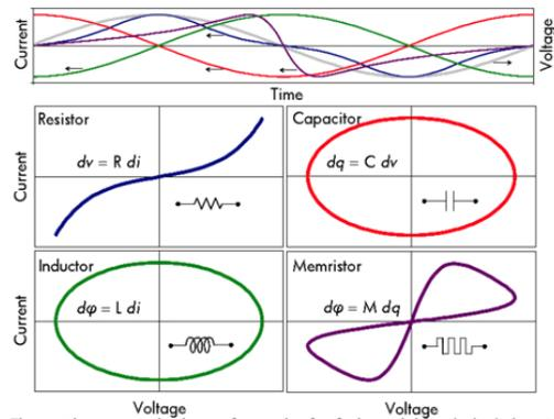
Fig. 2. The upper figure shows an applied voltage sine wave (gray) versus time with the corresponding current for a resistor (blue), capacitor (red), inductor (green), and memristor (purple). The lower figures show the current-voltage characteristics for the four basic circuit elements, with the characteristic pinched hysteresis loop of the memristor in the bottom right.
