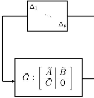
Fig. 1. The deviated system is represented as the interconnection between the structured uncertainty  $\Delta$  and the deterministic plant  $\tilde{G}$ . This separation allows us to test the MS stability of the system using the input-output maps of the mean system  $\tilde{G}$ .
