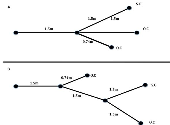
Fig. 6. Example of a star-shaped and tree-shaped networks
