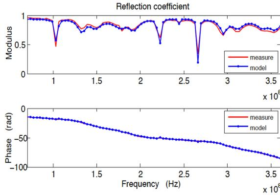
Fig. 8. Measured reflection coefficient compared to simulated reflection coefficient for a star shaped network.
