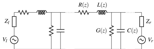
Fig. 1. A transmission line connected to a voltage source  $V_l$  with its internal impedance  $Z_l$  and to a voltage source  $V_r$  with its internal impedance  $Z_r$ .
