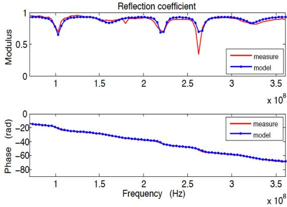
Fig. 7. Measured reflection coefficient compared to simulated reflection coefficient for a star shaped network.
