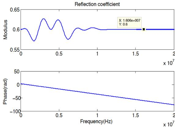
Fig. 4. Simulated reflection coefficient for a star shaped network
