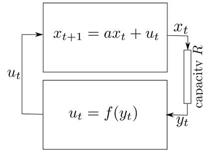
Fig. 1. A channel of capacity  $R$  restricts the communication between the plant and the controller. We look for the controller that will minimise a quadratic cost. The logarithmic strategy, which discretises  $x_t$  with a logarithmic quantiser, is shown to be suboptimal in the low capacity limit.
