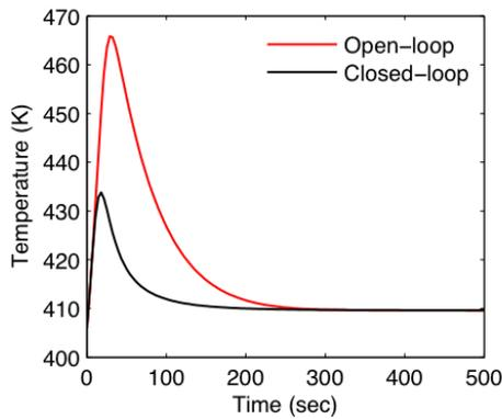
Fig. 5. Temperature response in the CSTR
