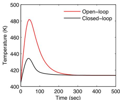
Fig. 7. Temperature response at the outlet of the PFR
