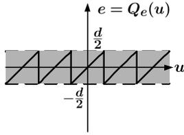
Fig. 4. Quantization error (Midtread type)
