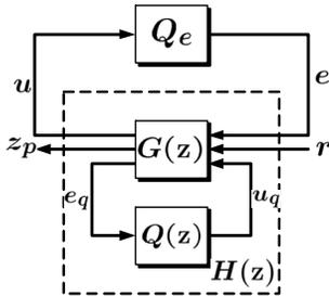
Fig. 5. Feedback system with quantization error
