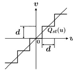
Fig. 3. Midtread type quantization
