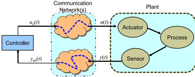
Fig. 1. Control over a network.
