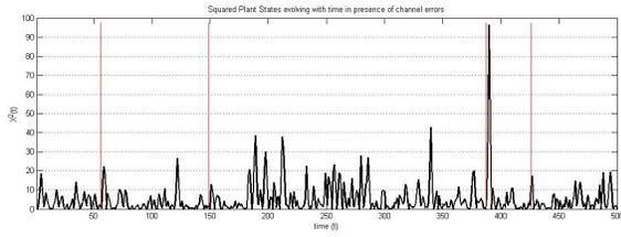
Fig. 1. Squared plant state  $X(t)^2$  vs. time  $t$ . The vertical lines indicate when symbol errors occur.
