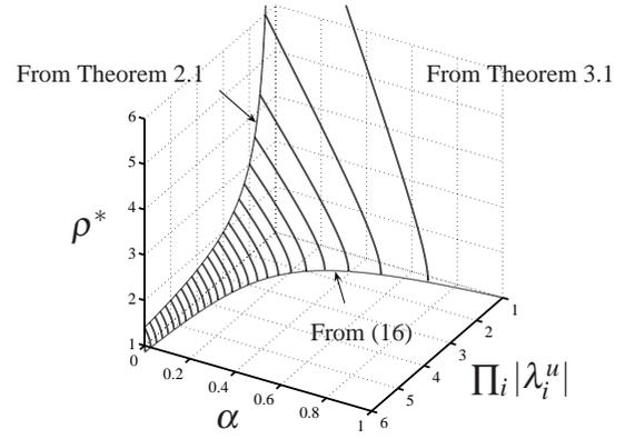
Fig. 5. The relationship between the product of unstable poles  $\prod_i |\lambda_i^u|$ , the loss probability  $\alpha$ , and the coarseness  $\rho^*$  of the quantizer.
