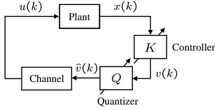
Fig. 8. Quantized adaptive control scheme
