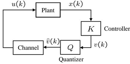
Fig. 1. Stabilization via coarsely quantized signals
