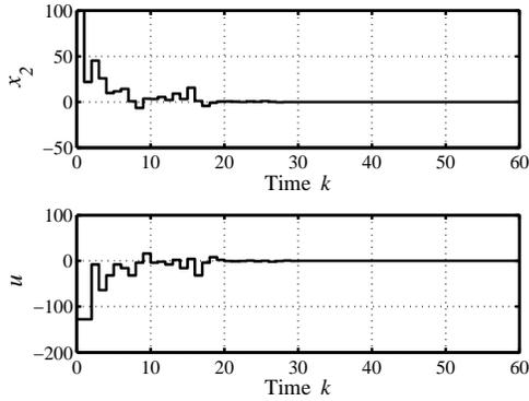
Fig. 6. Time responses of the system designed for the lossy channel: The state  $x_2$  (top) and the control input  $u$  (bottom)
