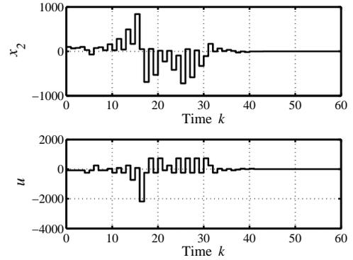
Fig. 7. Time responses of the system designed without accounting for the losses: The state  $x_2$  (top) and the control input  $u$  (bottom)
