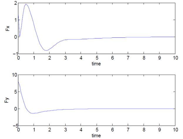
Fig(7): Simulations results of control inputs with  $Q=10, R=0.1$ .
