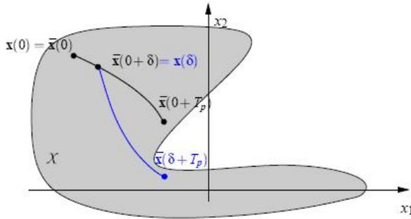
Fig(5): The difference between open-loop prediction and closed-loop behavior.
