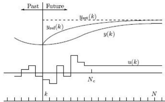
Fig(4): Principle of model predictive control.
