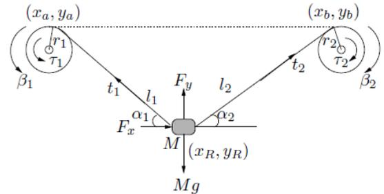
Fig. 3. Pulley-cable schematic
