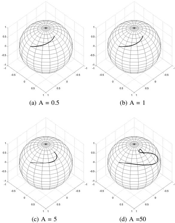
Fig. 4: Head movement to an arbitrary head position, under the influence of a potential function and a constant friction term. We have chosen  $\epsilon = 0.1$  and  $k = 1.0$ .
