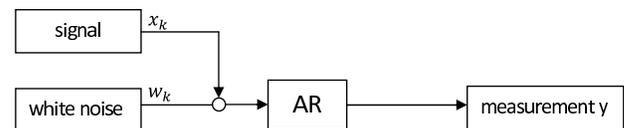
Fig. 1. Model for sinusoids in colored noise.
