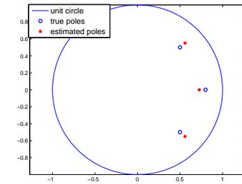
Fig. 8. Poles of true and estimated filters.
