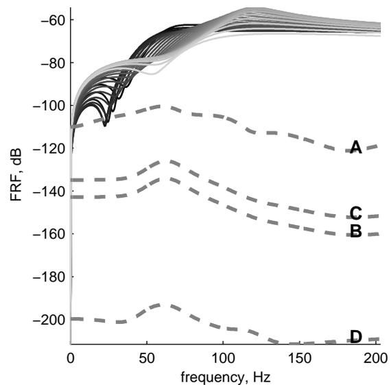
Fig. 6. Noiseless case: Evolution of the amplitude of the actual instantaneous FRF (gray shaded lines) of the simulated system. Grey dashed lines: RMS errors over all time instants of the estimated instantaneous FRFs.
