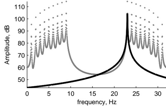
Fig. 4. Spectrum of sampled and windowed signal  $t \frac{dx}{dt}$ , zoomed out, with first repetition of the spectrum around the sample frequency. The first hyperbola in the repeated spectrum is shown explicitly (black full line).
