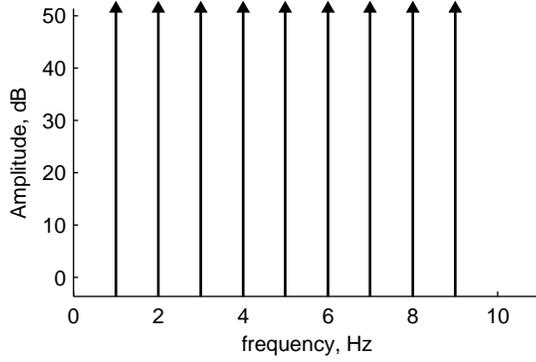
Fig. 1. Spectrum of a band-limited and periodic signal  $x$ .
