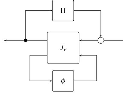
Fig. 2. Smith-predictor type structure
