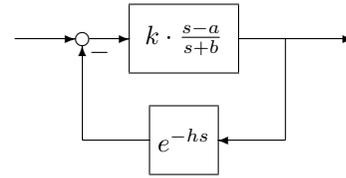
Fig. 5. Block diagram of a system with delayed feedback
