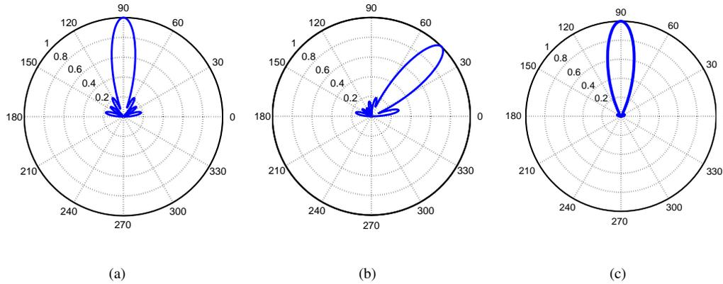
Fig. 4. (a): The radiation pattern obtained by maximizing the received power at the direction  $90^\circ$ ; (b): the radiation pattern obtained by maximizing the received power at the direction  $90^\circ$  subject to the constraints  $v_1 = v_2 = v_3 = v_4 = v_8 = v_9 = v_{10} = v_{11} = 0$ .
